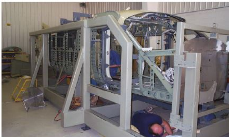
Mickey Stowers fabricated specialized fixtures to hold a Caravan fuselage in place, enabling ASIC technicians to rebuild any structural component on the aircraft.
