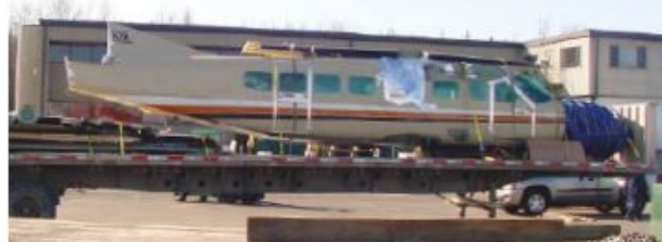
ASIC technicians travel all over the world to retrieve damaged Caravans. For shorter, drivable distances, they utilize a trailer with a special rack to transport the aircraft back to the shop.
